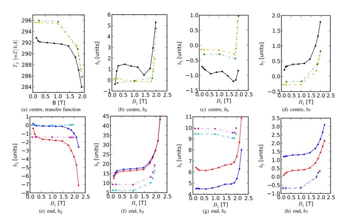
Figure 1: The measured (solid line) and calculated transfer function and harmonics versus the main field. centre: black – measured, yellow – TOSCA, green – ANSYS. end: connection side blue – measured, cyan – TOSCA; non connection side: red – measured, mangenta – TOSCA.
