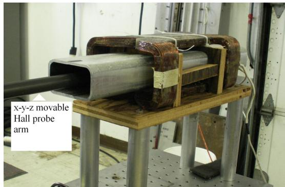
Figure 3: Measurement setup with air-core magnet.
