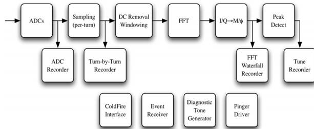
Figure 2: Block diagram of the tune measurement firmware.
