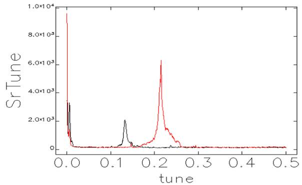
Figure 4: Storage ring tune plot (black trace: x tune, red trace: y tune).
