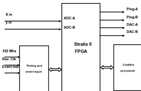
Figure 1: Block diagram of the tune measurement FPGA module.
