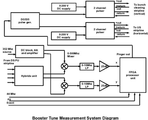
Figure 5: Block diagram of booster tune system.
