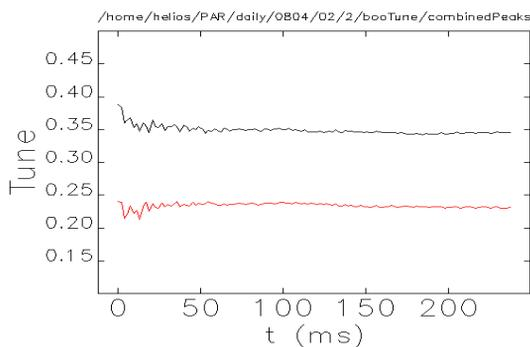
Figure 7: Peaks waveform of booster tunes (black trace: x tune, red trace: y tune).
