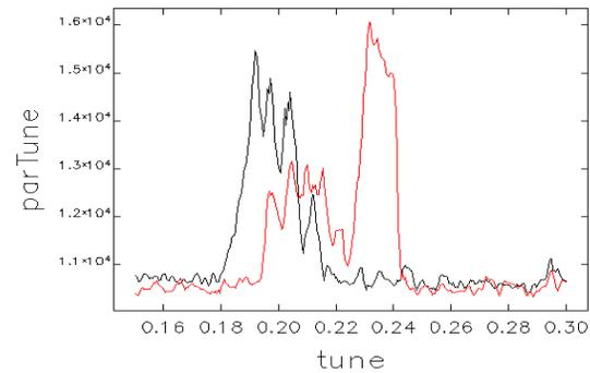
Figure 9: Plot of measured PAR tunes (black: x tune, red: y tune). The lower peaks are from injection perturbation.
