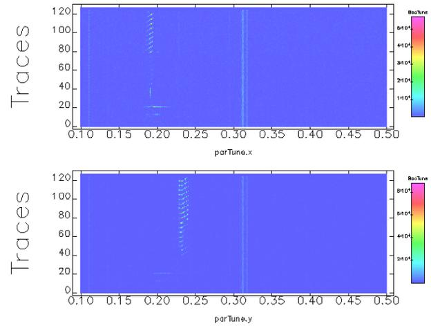
Figure 8: Contour plot of PAR tune history during a cycle (top: x tune, bottom: y tune).
