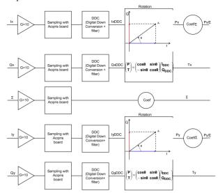
Figure 2: Schematic of signal post-processing.
