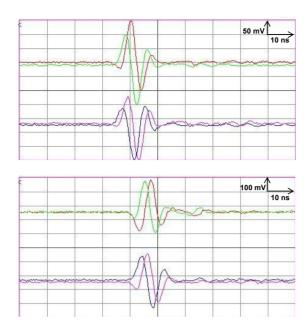
Figure 4: Visualisation of I and Q signals of two BPMs in vertical and horizontal frame in "10 bunches mode".
