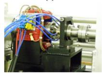
Figure 1: BPM and its steerer installed along the linac.
