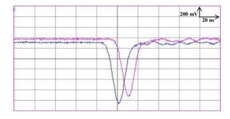
Figure 3: Visualisation of  $\Sigma$  signals of two BPMs.
