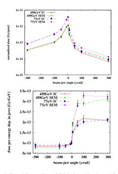
Figure 4: Top: Normalized BLM signal is plotted for a TCP collimator versus beam-jaw angle between  $\pm 300 \,\mu$ rad. Bottom: Ratio of BLM signal to total energy deposition in the jaws is plotted for a TCP collimator versus beam-jaw angle.
