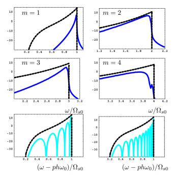
Figure 4: PD Schottky bands  $P/P_0$  for m = 1, 2, 3, 4(blue) for  $\Phi = \pi/8$ ,  $T_a = 320T_s$ . Bottom: dipole sideband (a.u.) in the traditional Schottky spectrum (cyan) for  $T_a = \infty$ , p = 5 (left, SPS 1 GHz system) and p = 12(right, LHC 4.8 GHz system). In all figures logarithmic scale (dB),  $2\Omega_{s0}/mF(\omega/m)$  as dashed line,  $\sigma_{\phi} = \pi/4$ .
