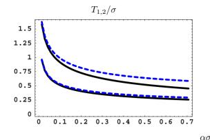
Figure 2:  $T_1/\sigma$  (dashed line) and  $T_2/\sigma$  (solid line) for  $\mu T_0 = 0.07$  (upper curves, SPS values) and  $\mu T_0 = 0.01$  (lower curves) found for a Gaussian line density.
