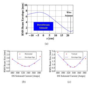
Figure 3: (a) Solution to the KV envelope equation using measured solenoid field profile. (b) and (c) Fitting to measured RMS beam sizes to obtain beam emittances.
