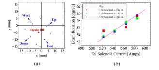
Figure 4: Beam rotation measurements. (a) Beam centroid for various dipole settings. (b) Comparison of measured beam rotation with calculations.
