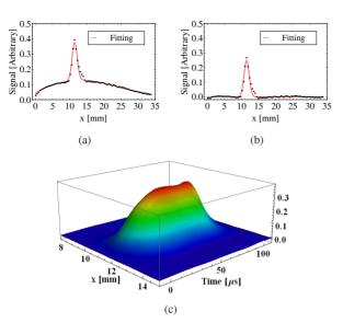
Figure 2: Beam profile measurement using wire scanner. (a) The fit has a R<sup>2</sup> value of larger than 0.99. (b) The fit is able to extract the profile of the proton beam from raw data. (c) The beam has a flat-top of about 50  $\mu$ s. For this measurement the RMS beam size is 0.64 mm ± 2%.
