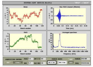
Figure 1: Positron grow-damp record made by switching off the horizontal feedback, I=575mA, 105/120 bunch [October 14, 2008].
