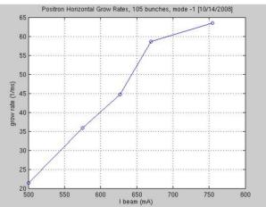
Figure 2: DAFNE e+ horizontal instability grow rate versus beam current [10/14/2009].
