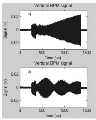
Figure 2: Signals from the wide-band BPM for coasting beam driven transversely at frequencies corresponding to the mode 20 lower sideband (a) and upper sideband (b). These signals are the difference signals from the top and bottom electrodes of the BPM, giving an indication of the vertical position of the beam. The drive was not present as the beam was accumulated during the first 100µs of the signal.
