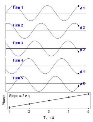
Figure 3: Illustration of the tune measurement technique. The first 5 plots show the transverse position of a slice of beam as it orbits the ring. The phase of its betatron oscillation is indicated after each turn. The bottom plot shows that the slope of the phase vs. turn gives the fractional part of the tune.
