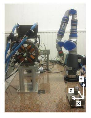
Figure 3: Platinum Faro arm and metal spheres defining the coordinate system.
