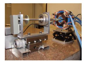
Figure 1: Rotating coil setup.
