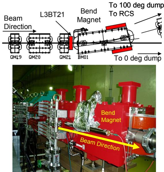
Figure 5: BLM installed at Bend Magnets.
