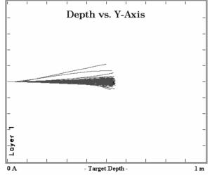
Figure 1: Plot of the stopping range of a 1-GeV beam in solid copper. The range of the horizontal axis is 1 m.
