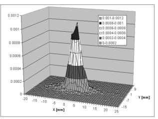
Figure 5: Plot of the beam intensity at the pickup 10 m downstream of the laser slit.
