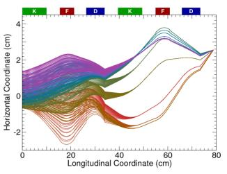
Figure 5: Injection of beams of various energies into EMMA. Energies are from 10 to 20 MeV in 1 MeV steps. Each color is a different energy: violet, toward the top, is the highest energy, and red, toward the bottom, is the lowest. For a given color, different lines are different initial conditions on the edge of an ellipse as in Fig. 3.
