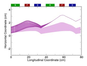
Figure 4: Injection of a 20 MeV beam into EMMA. Everything is as in Fig. 3, except only the 20 MeV circulating beam is shown.
