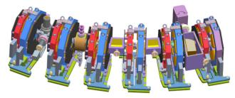
Figure 1: Injection region of EMMA, showing, right to left, the injection septum and two kickers.
