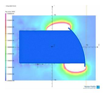
Figure 2: Septum, showing magnetic field magnitudes [5]. Transition to white is at 5 mT.
