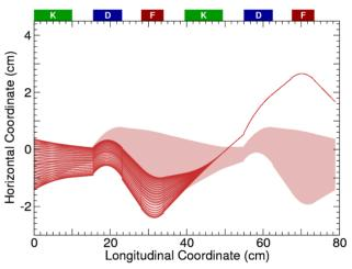
Figure 6: Extraction of 10 MeV beam from EMMA. The beam goes from left to right in the drawing. The last point plotted on the right is where the beam enters the septum. Only the 10 MeV circulating beam is shown. Everything else is as in Fig. 3.
