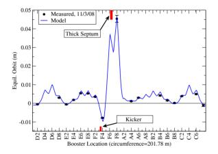
Figure 1: Booster extraction orbit distortion.
