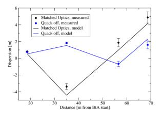
Figure 4: Dispersion measurements and model predictions.
