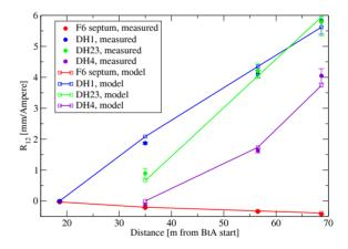
Figure 2:  $R_{12}$  measurements and model predictions; quadrupoles off case. Data is shown only at the four profile monitor locations. Error bars show the statistical spread of 5 to 10 independent measurements.
