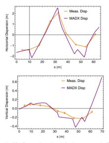
Figure 4: Horizontal and vertical measured dispersion in the transfer line shown with the theoretical dispersion from MADX with the stray field included in the simulation.
