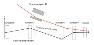
Figure 2: Layout of the PS injection.
