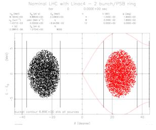
Figure 2: Bunches in the PSB at extraction.
