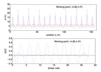
Figure 6: Betatron functions (upper image) and betabeating (lower image) with (solid) and without (dashed) active compensation of the perturbations introduced by the injection chicane. Red and blue traces denote horizontal and vertical phase space.
