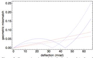
Figure 5: Geometric mismatch in the horizontal (red) and vertical (blue) phase space as function of the deflection during the fall of the chicane.
