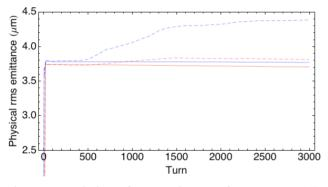
Figure 7: Evolution of rms emittances from ORBIT [6] simulations without and with active compensation.
