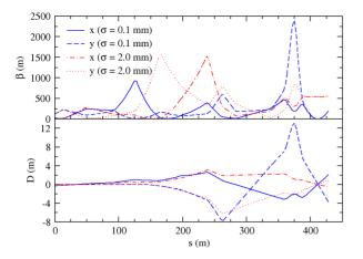
Figure 5: Simulated beta and dispersion functions for the TT61 solution for beam radii of 0.1 and 2.0 mm at the target.
