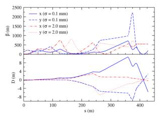
Figure 3: Simulated beta and dispersion functions for the T9 solution for beam radii of 0.1 and 2.0 mm at the target.
