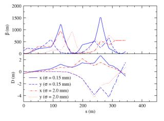
Figure 4: Simulated beta and dispersion functions for the T1 solution for beam radii of 0.15 and 2.0 mm at the target.
