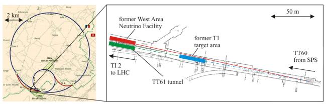
Figure 1: Possible locations of HiRadMat: The former West Area Neutrino Facility (red), the former T1 target area (blue) and the TT61 tunnel (green).
