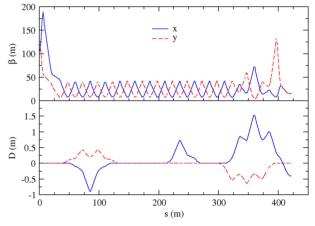
Figure 3: Simulated beta and dispersion functions along the SPL-PS2 transfer line for a 4 GeV  $H^{-}$  beam using MAD-X.
