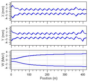
Figure 4: Envelopes in the horizontal (top) and vertical (middle) planes plus the beam energy spread (bottom) evolution along the beam line with a current of 62 mA.
