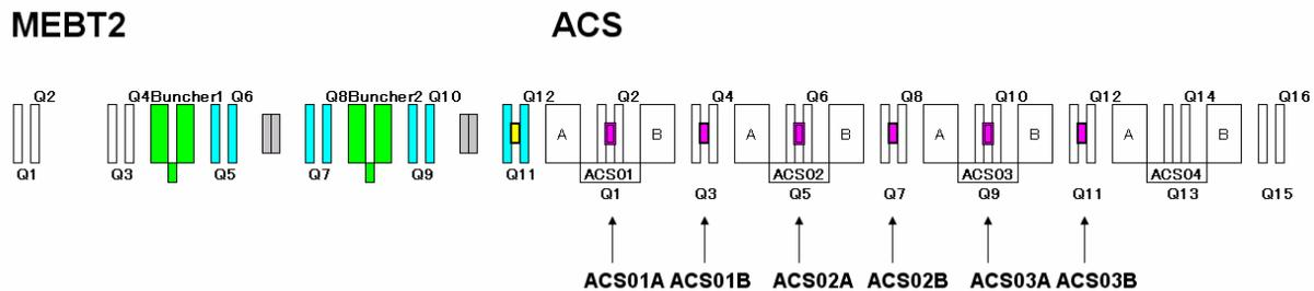
Figure 1: A schematic layout of MEBT2 and the beginning of ACS. The geometry is not to scale. Magenta rectangles show candidate positions for WSMs and BSMs.
