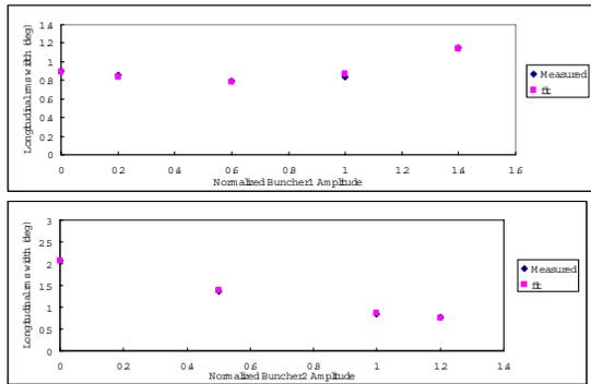
Figure 5: “Measured” (blue) and fitted (magenta) longitudinal widths as a function of amplitudes of Bunchers 1 (top) and 2 (bottom) in Scheme B for ACS01A.
