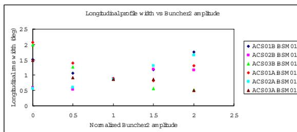
Figure 3: Longitudinal profile width in degrees of 324 MHz as a function of Buncher 2 amplitude.
