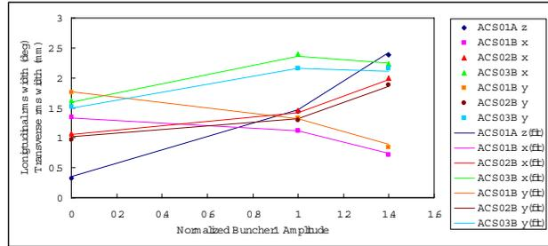
Figure 6: “Measured” (symbols) and fitted (lines) longitudinal and transverse profile widths in Scheme C for ACS01A.
