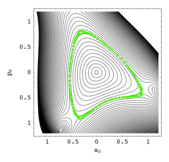
Figure 2: Invariant contours from  $|\phi_0|$  for Henon map compared to tracking results (green).
