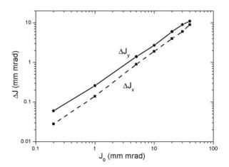
Figure 6: Variation of action amplitude versus beam emittance.
