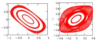
Figure 3: X (left) and Y phase spaces for 25 percent beta-function difference. (19) and  $\beta=1.25$ .
