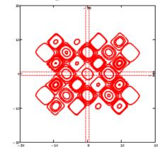
Figure 2: Phase space of the 1-cell map with periodic integrable lens.
