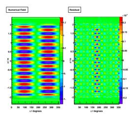
Figure 2: Left: The  $B_{\rho}$  component of the magnetic field on the surface of a cylinder for the CESR-c wiggler. This field is used to calculate the generalised gradients at any point within the cylinder. Right: The residual field of the input field (left) and that calculated using the generalised gradients on the surface of the cylinder.
