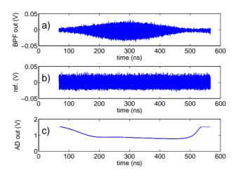
Figure 4: Preliminary test of the phase detector at the AWA. The beam induced signal downstream of the 1.3 GHz BPF (a) is compared to the 1.3 GHz reference signal (b) in a Analog Device chip whose output voltage (c) is proportional to the phase difference between the beam-induced and reference signals.
