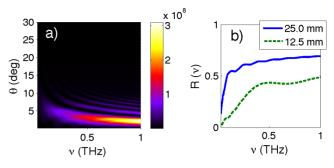
Figure 5: Transition radiation generated by a 5 GeV electron in the sub-mm wavelength regime. Left plot: spectral spectral radiance with a 25 mm foil at observation distance R = 15.24 cm ( $\simeq 6$ "). Right plot: acceptance ratios  $R(\nu)$  of viewing windows of 12.5 mm and 25.0 mm radius at a distance of 15.2 cm from the emission source.
