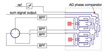
Figure 3: Block diagram of the phase detector assembly. The four signals from a beam position monitor (BPM) are filtered with 1.3 GHz band pass filter (BPF) and compared with the reference signal to yield the phase. The sum/comparison is performed in a rf printed circuit board.
