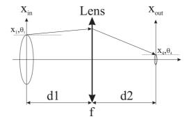
Figure 3: General geometry of one diagnostic Station of the ATF-II laser-wire LTL.
