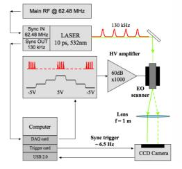
Figure 3. Experimental setup.
