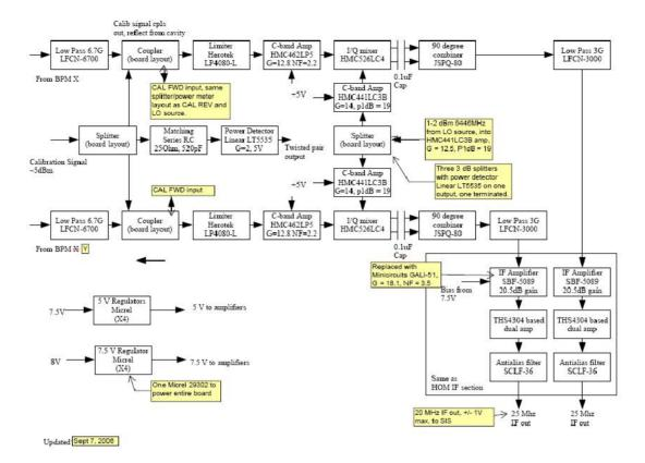
Figure 2: Schematic of the BPM downmix electronics.
