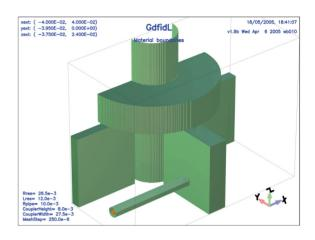
Figure 1: Design of the ATF2 C-Band cavity shown in the format used for the GdfidL simulations.
