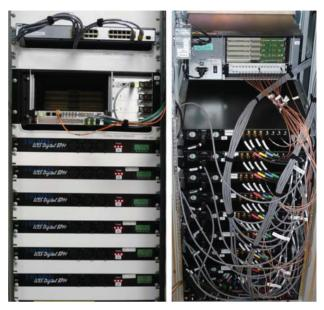
Figure 7: BPM processors in the rack, front and back.
