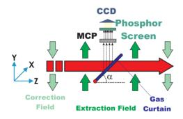
Figure 3: Gas curtain monitor working principle.
