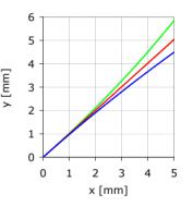
Figure 2: Disturbance of different primary beams in the presence of the SEE monitor: 20 keV antiprotons (green), 300 keV antiprotons (red) and 20 keV protons (blue).
