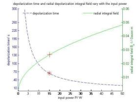
Figure 1: The depolarization time and the radial integral field vary with the input power.
