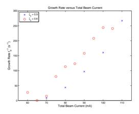
Figure 6: Mode 360 growth rate versus current, for vertical chromaticities of 0.9 and 0.6.
