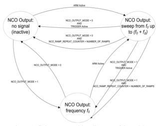
Figure 1: finite state machine diagram of the NCO.
