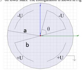
Figure 2: The configuration of kicker. It has four electrodes mounted in a skew 45°.
