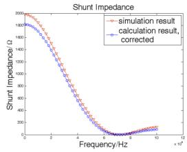
Figure 5: The corrected calculation shunt impedance curve and the simulation result.
