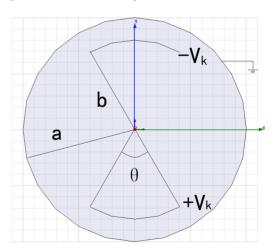
Figure 1: The configuration of y-kicker of two electrodes.
