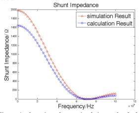
Figure 4: shunt impedance: simulation and calculation results.
