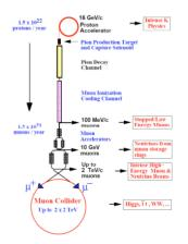
Figure 1: Schematic of MC subsystems.
