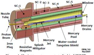
Figure 4: Hg-jet target concept studied in MERIT.
