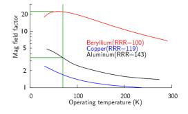
Figure 8: Relative increase in allowable axial field vs. initial temperature for Copper, Aluminum, and Beryllium.
