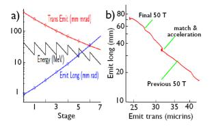
Figure 6: a) Energy, longitudinal, and transverse, emittances for 7 stages of final cooling; b) Long. vs. trans. emittances through the last two stages including matching and re-acceleration.
