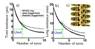
Figure 4: Simulation of a) transverse, & b) longitudinal, cooling in RFOFO 6D lattice; c) Cooling geometry.
