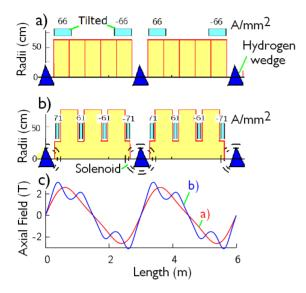
Figure 10: a) Two cells of a conventional RFOFO lattice; b) a magnetically insulated version of the same; and c) the magnetic fields vs length in the two cases.
