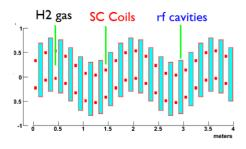
Figure 5: An example of a Helical Cooling Channel.
