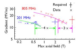
Figure 7: Observed breakdown gradients vs maximum axial fields on cavities, together with approximate required gradients: 201 MHz in blue, 805 MHz in red.
