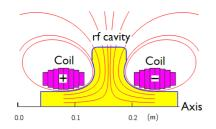
Figure 9: Magnetically insulated cavity with magnetic fields parallel to surfaces.
