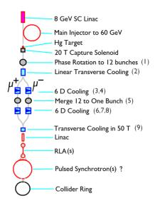
Figure 1: Schematic of Muon Collider components.
