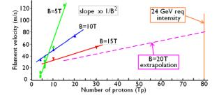
Figure 2: MERIT observed filament velocities vs. proton intensity at B=5, 10, 15 T, & dashed extrapolation to 20 T.
