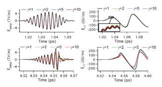
Figure 3: History of perpendicular (left) and longitudinal (right) electric field at the positions (in the laboratory frame) x = y = 0,  $z_1 = 0.154mm$  (top) and  $z_2 = 1.354mm$  (bottom) from simulations in the laboratory frame (black) and boosted frames at  $\gamma_f = 2$  (green), 5 (blue), and 10 (red).
