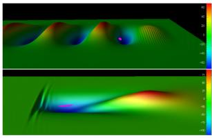
Figure 2: Colored surface rendering of the longitudinal electric field from a 2-1/2D Warp simulation of a laser wakefield acceleration stage in the laboratory frame (top) and a boosted frame at  $\gamma_f = 10$  (bottom), with the beam (magenta) in its early phase of acceleration.
