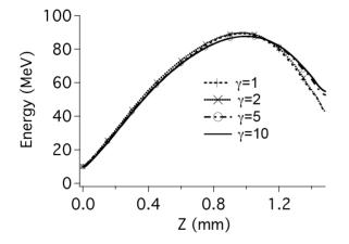
Figure 4: Average beam energy versus longitudinal position in the laboratory frame from calculations in a frame moving at  $\gamma_f = 1, 2, 5$  and 10.
