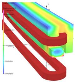
Figure 3: Magnetic model of the upper half of the yoke (and upper & lower coils) with optimized "nose" piece.
