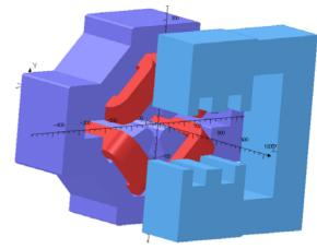
Figure 7: Magnetic model used for studying interaction harmonics between SLS quadrupole and NSLS-II 156 mm prototype corrector dipole. The corrector dipole is not powered and the coils are not shown.
