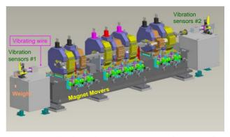
Figure 14: Vibrating wire system at BNL for measuring and adjusting centers of sextupoles and quadrupoles.
