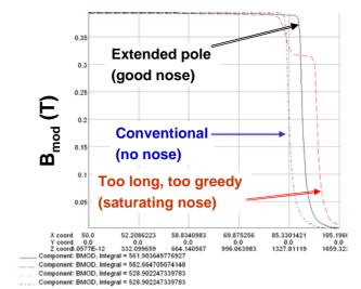
Figure 5: Dipole field (magnitude) along the beam axis from the middle of the dipole in these three cases.
