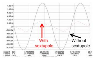
Figure 12: Radial component of the field as a function of angle at R=25 mm in a plane perpendicular to the magnet axis at the location where the sextupole iron starts.
