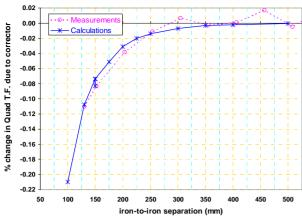
Figure 9: Comparison between calculations and measurements for the drop in integral quadrupole transfer function due to the presence of the corrector dipole (not powered) as a function of yoke-to-yoke separation between the two magnets.
