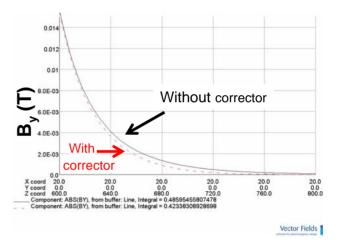
Figure 8: Vertical field component  $(B_y)$  parallel to magnet axis (x=20 mm, y=0 mm) outside SLS quadrupole without and with NSLS-II corrector dipole in proximity (yoke-to-yoke gap=130 mm).
