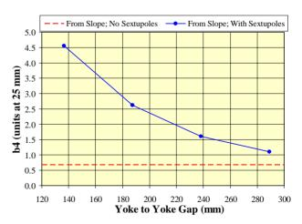
Figure 13: Measured integral octupole ( $b_4$ ) harmonic in quadrupole as a function of yoke-to-yoke gap when a sextupole (not powered) is placed in the vicinity (blue solid line). Inherent  $b_4$  is shown by red dashed line.
