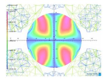
Figure 11: Contour plot of the magnitude of the radial component of the field in a plane perpendicular to the magnet axis at the location where the sextupole iron starts. The poles of the quadrupole and sextupole are projected here. Only the quadrupole is powered.
