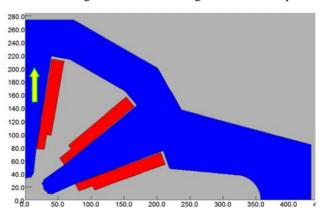
Figure 6: Magnetic model of a quadrant of the 68 mm aperture wide sextupole for NSLS-II. Poles must be moved vertically away from the center (see arrow) to compensate for the break in symmetry caused by a large cut-out in the iron yoke to allow X-ray transport.
