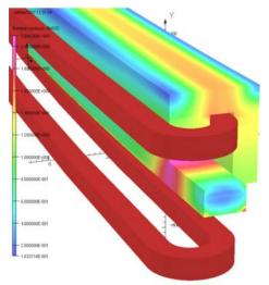
Figure 4: Magnetic model of the upper half of the yoke (and upper and lower coils) with a "nose" piece that is too long and causes saturation.
