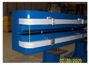
Figure 1: Prototype magnet for NSLS-II with "extended pole" or "nose". The dotted line shows the boundary between the nose piece and the main laminations.
