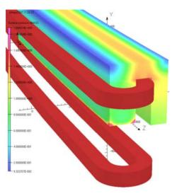
Figure 2: Magnetic model of the upper half of the yoke (and upper and lower coils) without "nose" piece.
