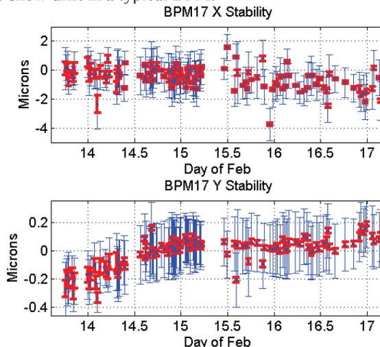
Figure 6: Position stability for a BPM over days. Each dot is the mean measured position for ~100 pulses after beam jitter removal. Blue error bars represent the rms spread of position, red bars are the expected error of the mean.
