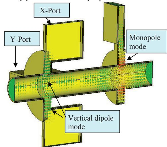
Figure 1: BPM Cavity schematic with electric fields of position (dipole) and reference (monopole) cavities.
