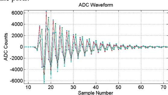
Figure 3: BPM raw waveforms sampled at 119 MHz.
