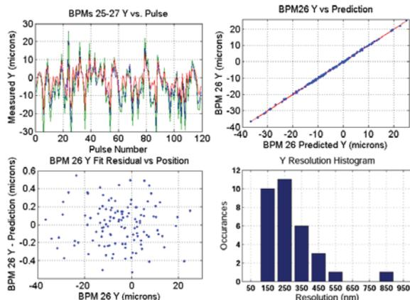
Figure 5: Upper-left: Y position measured at adjacent BPMs for 120 pulses. Upper right: Y at BPM26 vs. best fit prediction from its neighbors. Lower left: Fit residual, Lower right: Histogram of measured BPM resolutions.
