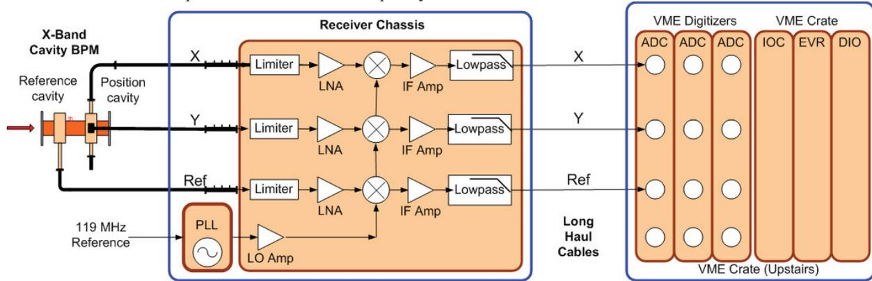
Figure 2: System block diagram. The receiver is mounted on the undulator stand while the digitizers are upstairs.
