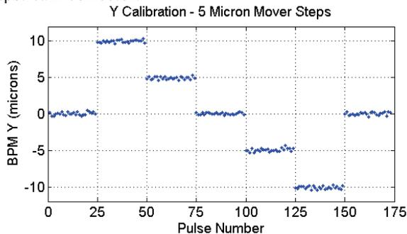
Figure 4: Calibration moving BPM in 5 micron steps.
