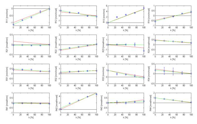
Figure 2: Measurement of the A0 emittance exchanger transport matrix as a function of the deflecting cavity strength k in units of the ideal cavity strength ( $k_{ideal}$ ). The green line is a fit to the data. The red line is the prediction.[13,14].
