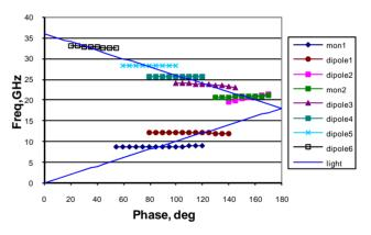
Figure 1: Dispersion curves for the 2 monopole (blue, green) and 6 dipole modes in the CLIC crab cavity.
