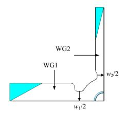
Figure 4: Four-port waveguide damper.
