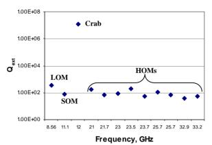
Figure 5: Q<sub>ext</sub>'s of the modes in a waveguide-damped cavity.
