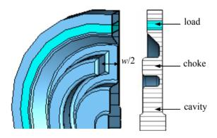
Figure 2: Asymmetric choke-mode cavity.
