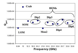
Figure 3: Q<sub>ext</sub>'s of the modes in an asymmetrical chokedamped cavity. (degenerate modes are encircled).
