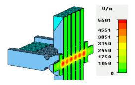
Figure 6: A 7-cell damped travelling wave crab cavity.
