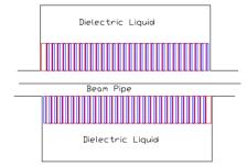
Figure 3: Dielectric Loaded Cavity for Phase Rotation
