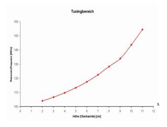
Figure 3: Frequency range (x-axis: Tuning plate height).
