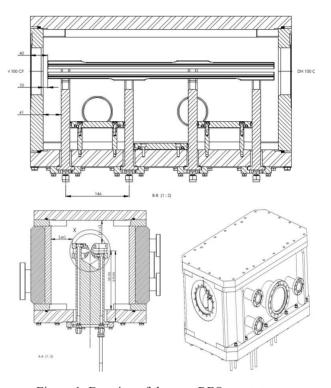
Figure 1: Drawing of the new RFQ- prototype.
