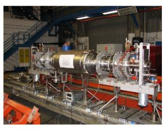
Figure 1: The ERL accelerating cavity hermetic string assembly shown before installation into the cryomodule.
