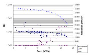
Figure 4: The preliminary test data from the cryomodule including radiation measurements presented along with the previous VTA measurements.
