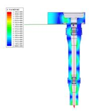
Figure 2: E-filed of the KEK STF baseline high power input coupler with two choke structures.
