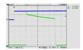
Figure 4: Pulse of the 12 kV solid switch cell module.
