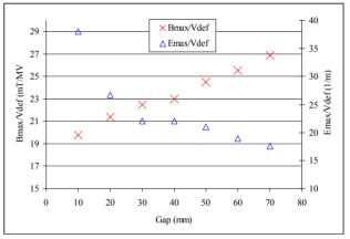
Figure 2: Plot of  $E_{max}/V_{def}$  and  $B_{max}/V_{def}$  at various Rod gaps
