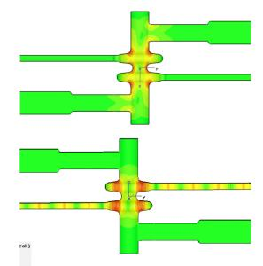
Figure 1: H magnitude plot for the operating mode (top) and E magnitude plot for the SOM (bottom)
