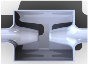
Figure 4: Cut away of cavity shape showing 2 facing rods.
