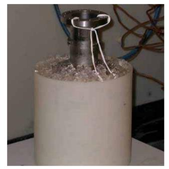
Figure 1: BCP of a single-cell Niowave cavity packed in ice. The white Teflon rope supports a Niobium sample inside the cavity for material removal measurements.
