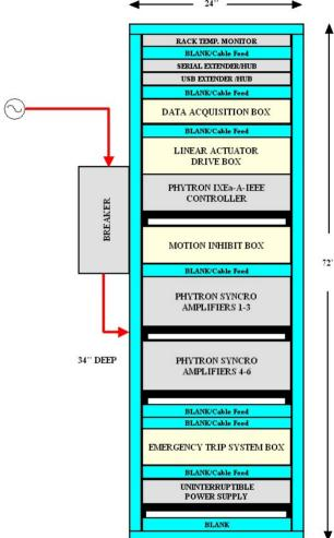
Figure 2: Control Rack Layout.
