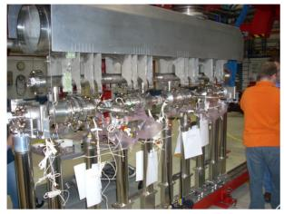
Figure 3: Completed string assembly .
