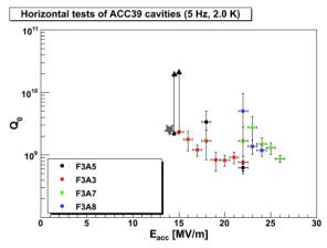
Figure 1:  $Q_0$  vs E for the 4 cavities in the String assembly. The star indicates the design goal.
