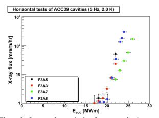
Figure 2: Onset and magnitude of x-ray production as a function of gradient.
