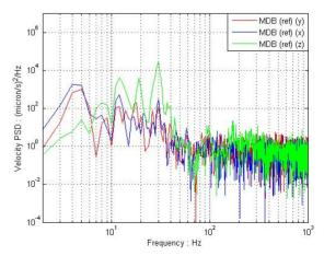
Figure 6: Velocity PSD baseline for MDB.
