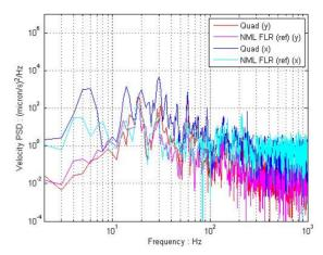
Figure 4: Velocity PSD baseline for NML.
