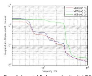
Figure 5: Integrated displacement baseline for MDB.
